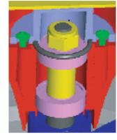
Labyrinth seal, o-ring attached top cap
